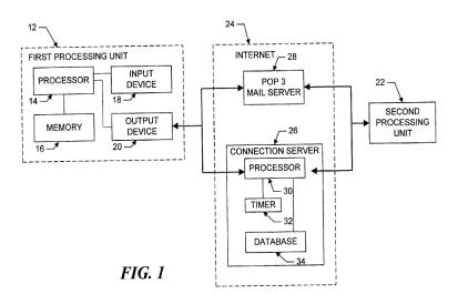
Figure 1 above illustrates the architecture between first processing unit 12, second processing unit 22, and connection server 26. *Id.* at 6:50–64.
